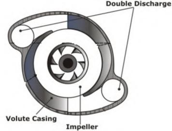
This figure show how the thrust is balanced by the Twin-Volute with 180 degrees opposite discharge outlets.
